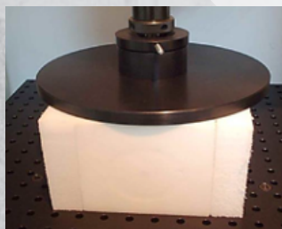
Compression test. \sigma_m = 255 \text{ kPa}
